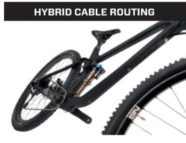
The cables appear to be threaded through the downtube and chainstay... But actually, they are only hidden in a special channel in the construction. Easy to replace anytime, anywhere!
